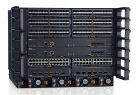
The C9010 Network Director is based on the new Dell campus network architecture. It is a multi-rate capable modular switch scalable for up to 4000 virtual ports, with support for 10 and 40GbE and a future tool-free upgrade to 100GbE.
