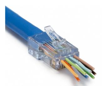
It features the same unique patented Hi-Lo stagger load bar, allowing conductors to pass through the front end of the connector to easily verify the wiring sequence before termination. The insulation diameter of the conductor is 0.84-0.97mm, while the maximum outer diameter is 7.36mm.
