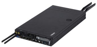
According to the company, the SE350 allows for reliable server-class performance at many Edge locations. The rugged design handles temperatures from 0° to 55°C, and also tolerates locations with high dust and vibration, such as construction site trailers and manufacturing floors. Office-friendly acoustics allow deployment in traditional office or branch locations.
