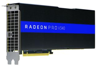
Based on Vega architecture, the V340 is the first AMD VDI hardware solution equipped with 32GB of 2nd generation high-bandwidth memory. Powering it are GPUs built using the 14nm FinFET process, as paired with AMD MxGPU hardware-based GPU virtualisation technology, which in turn is based on industry standard SR-IOV (Single Root I/O Virtualisation) technology.
