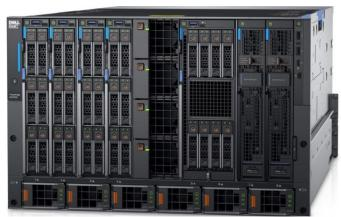
The design of the MX has no mid-plane, allowing support for fully disaggregated components, down to memory-centric devices such as storage-class memory, GPUs and FPGAs. As a result it offers full composability, transforming infrastructure into a "dynamic pool of instantly responding, adapting and evolving resources."
