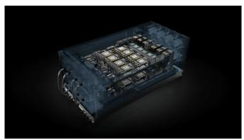
According to the company, the HGX-2 is "the first unified computing platform for both artificial intelligence and high performance computing." It offers up to 2 petaFLOPS performance for low-precision tensor operations, 250 teraFLOPS at single-precision and 125 teraFLOPS for double-precision.
