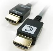
The cables offer a low smoke and fire-retardant plenum jacket, as well as UHD, 18G 4K 60 4:4:4 end to end performance, with high-speed, plug-and-play HDMI signal transmission in lengths of up to 33m. Active components in the connectors perform electrical-to-optical conversion, drawing power from the HDMI port.
