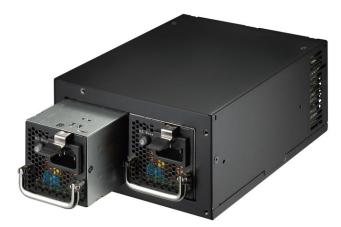
The two Twin Series modules differ in one wattage output, as one unit is rated at 500W and the other at 700W. Each contains two independent power modules with an own power adapter. During regular operation the two modules share the load for maximum efficiency and stability, but should one fail the other automatically takes over as "a clean fail safe." Hot-swap functionality allows the easy swapping of PSU modules without any downtime.
