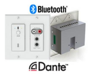
Included with the unBT2A, Attero Tech's **unBT2A EXP expander unit** provides balanced mono or stereo analog audio output on three-pin depluggable connectors, enabling easy connection to the audio system. The outputs are software switchable between -10 dBV (consumer) and +4 dBu (professional) nominal output levels. The unBT2A EXP sports an RS-232 port for third-party control and customization, using a simple serial protocol.
