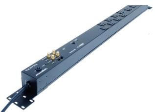
The VT4315 Pro mounts vertically on the back of equipment, and leverages on BlueBOLT IP control technology to control 12 outlets in 8 banks (4 individually controlled outlets and 8 in paired duplex banks). As Panamax puts it, such a configuration enables remote monitoring and reboot in either real-time or via scheduled commands from the connected equipment in the rack.
