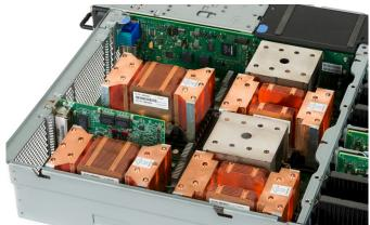
The flagship refreshed offering is the S822LC. It features 2 Prower8 processors complete with PowerAccel interconnects including NVLink, a proprietary connector for high-speed connection with Nvidia Tesla P100 Pascal GPUs. The NVLink is embedded at silicon level to enable data speeds up to 5x faster than on x86-based systems.
