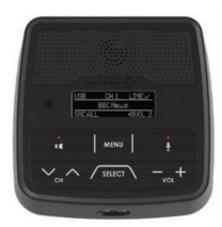
Attero Tech's **Dante unDNEMO** is an audio monitoring solution providing end users with a simple solution for selection and monitoring of up to 64 Dante audio channels.
