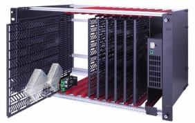
As the company puts it, the ONErack converts randomly sized, externally powered devices from all vendors into easy installable slide-in modules. The rack has both front and rear access, provides uniform cable management and allows for high density mounting with 3 different chassis sizes, 7 different voltages and cooling.
