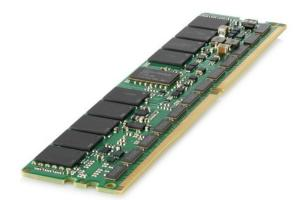
Dubbed NVDIMM (Non-Volatile Dual In-Line Memory Module), the technology pairs 8GB of DRAM with 8GB of NAND flash. As well as persistence and performance, HPE says Persistent Memory ensures no data is lost from the memory module in case of power outage, since the flash backs up all DRAM contents while a Smart Storage Battery (with support for up to 16 NCVDIMMs) provides backup power.
