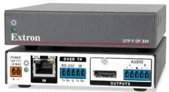
The two devices extend signals for up to 70m or 100m, and both provide an effective means for incorporating higher resolution DisplayPort signals with embedded audio into Extron DTP systems. Video resolution support reaches 4K with simultaneous analog stereo audio signal transmission over the same shield twisted pair cable.
