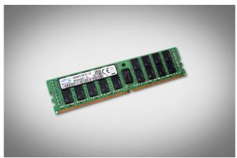
An update on the 64GB TSV DDR4 DRAM modules introduced in 2014, the new Samsung TSV DRAM modules claim the largest capacity and highest neergy efficiency around, while offering high speeds and "excellent" reliability. Each 128GB TSV DDR4 RDIMM carries 144 DDR4 chips arranged into 36 4GB DRAM packages. Each package in turn contains four 20nm-based 8Gb chips assembled using TSV packaging technology.
