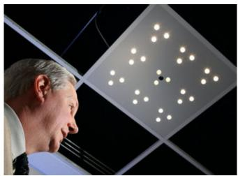
LED clusters in a ceiling light fixture transmit messages by flickering faster than the eye can see. Special modems "read" the messages and flicker messages back to the fixture's sensor-connecting a computer to the internet.
