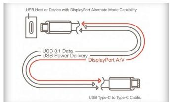
Essentially, Alt Mode adds DisplayPort capabilities to USB Type-C connectors and cables, allowing them the carrying of video signals (up to 4K), SuperSpeed USB (USB 3.1) data and up to 100W of power. It will also feature adapters to support existing DisplayPort, HDMI, DVI and VGA displays.
