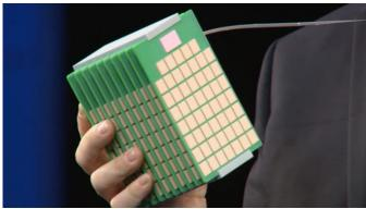
In a few words, The Machine consists of clusters of special-purpose cores, with silicon photonics (ie lasers) replacing traditional copper wires. Serving as both memory and storage are <a href="memristors">memristors</a>, a futuristic technology as fast as RAM yet also able to store data permanently, while tying all together is a new free and open source Machine OS.
