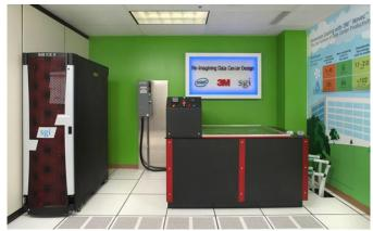
The machine consists of an an Intel Xeon E5-2600-powered SGI ICE X supercomputer submerged "Novec Engineered Fluid", a liquid 3M describes as "an efficient dielectric that keeps the hardware cooled with minimum additional energy, maximum performance and better reliability."
