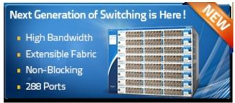
The company says the switch offers non-blocking connectivity of 288 10G signals for total 2.88Tbps throughput. It promises 100% network visibility, with redundancy, high availability and an extensible backplane.
