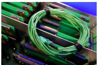
The cables push 25Gbps of data across each fibre, and were first seen last year with speeds reaching 100Gbps. The connectors are called "MXC," an Intel-Corning development holding up to 64 fibres (32 up, 32 down) to allow the aforementioned 800Gbps connection speeds-- even if Intel prefers to speak of a "1.6Tbps" aggregate.
