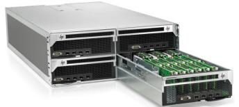
The launch follows 18 months of development since the November 2011 announcement of Project Moonshot. It was first revealed as "Redstone," an ARM-based design packing either 288 EnergyCards (a Calxeda reference design packing x4 EnergyCore SoCs, x4 DIMM slots and x4 SATA slots on a single daughterboard) on a 4U rack-mount server or 2800 on a full rack, together with shared power, cooling and management infrastructure.
