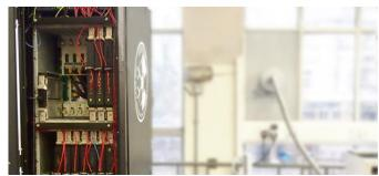
"Wet" computing is a fairly simple concept. A single Iceotope Platform rack holds up to 48 hot-swappable server modules, each being a self-contained aluminium unit holding server components submerged in Novec, an inert liquid coolant from 3M.
