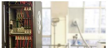
"Wet" computing is a fairly simple concept. A single Iceotope Platform rack holds up to 48 hot-swappable server modules, each being a self-contained aluminium unit holding server components submerged in Novec, an inert liquid coolant from 3M.
