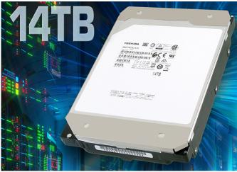
The MG07ACA comes in 14TB 9-disk and 12TB 8-disk models. According to the company, the helium-sealed 3.5-inch mechanical design allows for better storage density and a lower HDD operating power profile than the previous MG06ACA series. Laser welding technology ensures the helium remains sealed inside the enclosure.
