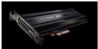
Aimed for datacentre use, the P4800X is ideal for high read/write applications demanding low latency, It has sequential transfer speeds of 2400MB/s read and 2000MB/s write, and can sustain high IOPS of 550000 read and 500000 write even at low queue depths. The result allows customers to do more work with the same servers, improving TCO or expanding capabilities, Intel claims.
