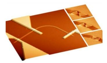
The company recently announced it has a working Racetrack Memory circuit at the IEEE International Electron Devices conference, with a chip consisting of 256 Racetrack "cells." Each cell consists of a nanowire 240nm wide and 20nm thick, with "spin currents" (electric currents, in other words) manipulating the magnetic state of the nano-scale magnetic regions within the nanowires.
