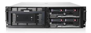
The system can store up to 768TB in a single chassis, with backup or restore data speeds of up to 28TB per hour. It scales from 48TB (one node with no expansion unit) to 768TB (fully loaded 4-node configuration), with a deduplication ratio of around 20:1.
