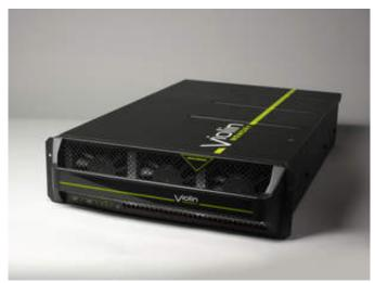
Everything comes in twos inside the 6000 series-- dual controllers, power supplies, gateway ports, even extra Violin virtual memory modules (VIMMs) providing self-healing and memory aggregation.
