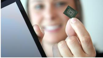
SanDisk and Toshiba's developments in NAND flash memory get even smaller-- producing a 64Gb X2-based monolithic chip with 19nm technology.
