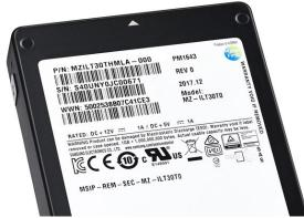
Aimed for enterprise systems, the PM1643 doubles the capacity of the previous 15.36TB Samsung SSD through the combination of 32 new 1TB NAND flash packages. Each package is comprised of 16 stacked layers of 512Gb V-NAND chips, and allows the storage of approximately 5700 5GB HD movie files in a 2.5-inch device.
