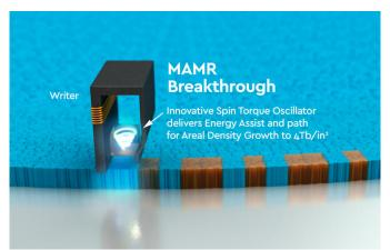
MAMR promises "all the gain without the gain" of the other energy-assisted HDD technology, heat-assisted magnetic recording (HAMR). According to WD, MAMR manages such a breakthrough through a "spin torque oscillator," a means to generate a microwave field able to increase the ability to record data at ultra-high density without sacrificing reliability.
