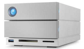
Featuring a chassis designed by Neil Poulton, the 2big features a single cable to connect with laptops, SD cards, compact flash cards and other devices. It handles up to 20TB of storage (a 25% increase over the previous version), while Thunderbolt 3 allows transfer speeds of up to 440MB/s.
