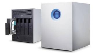
The 5-slot 5big arrays feature dual-Thunderbolt 2 connectivity and hardware RAID, allowing support for 4K video workflows. Bandwidth reaches up to 11050MB/sec, while the enterprise-class HDDs offer speeds of up to 7200rpm. LaCie says such bandwidth is enough for Adobe Premiere or Final Cut Pro users working on multiple 4K video streams in real time.
