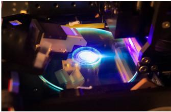
According to the company holographic storage is more robust than tape storage, while featuring the benefits of random access storage. It ships as removable optical media, meaning it is as easy and familiar to use as DVDs, with a small footprint, low costs and low energy consumption.
