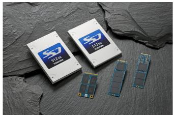
The HG6 drives are the first to use Toshiba 19nm MLC NAND flash, and carry the company's own controller and firmware. The interface of choice is SATA-6Gb/s, and form factors include 2.5-inch (7/9mm heights), mSATA and M.2 (single-sided, dual-sided).
