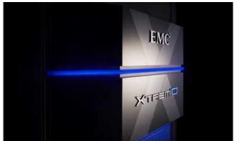
The XtremIO is based on modules EMC calls "X-Bricks." Available in 10TB capacities (20TB to follow in 2014), X-Bricks carry 256GB of RAM, and customers can cluster up to 4 together, with in-line deduplication allowing the configuration of around 250TB of effective capacity within a single cluster and performance reaching 1 million IOs per second.
