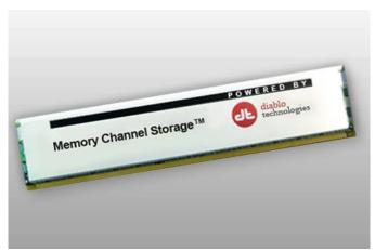
In a few words, MCS uses the standard DDR-3 CPU interface and protocols to connect flash storage to the CPU instead of RAM. Thus it takes advantage of the fastest route to the CPU, and makes use of multiple parallel DIMMs (dual in-line memory modules) to avoid bottlenecks.
