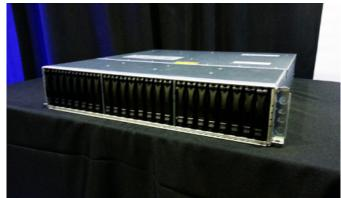
It carries up to 19.2TB of storage in a 2U rack-mount space and delivers over 300000 IOPS with sub-millisecond latency. Built on the SANtricity OS, the EF540 is complete with fully redundant components and takes seconds to carry out out backups and disaster recovery.
